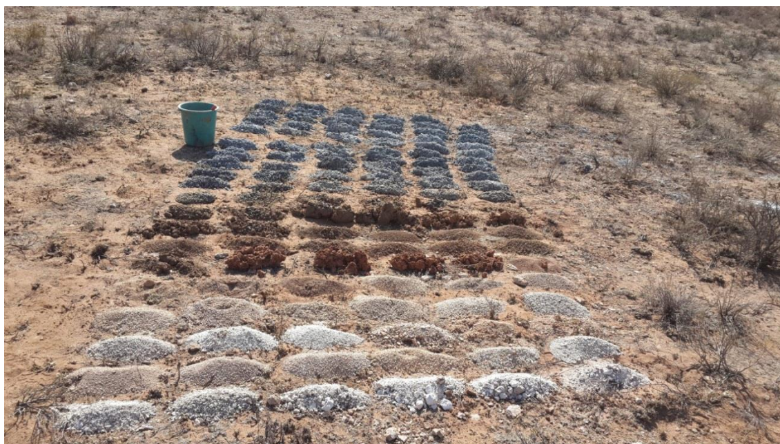
Figure 26: SD2-8 Borehole Drill Samples/Cuttings
